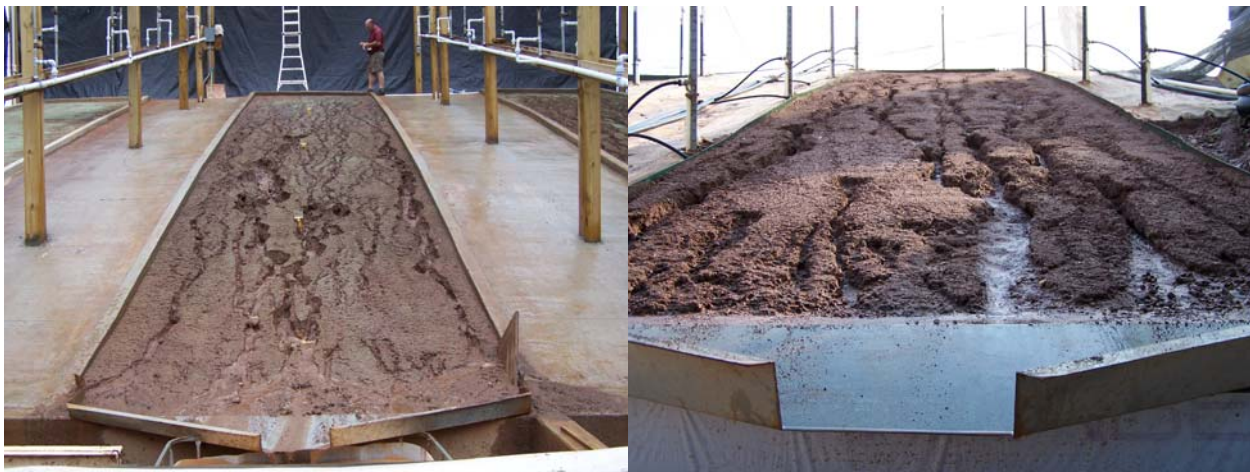
Figure 5. Test Slope #2 – Upon Test Completion
